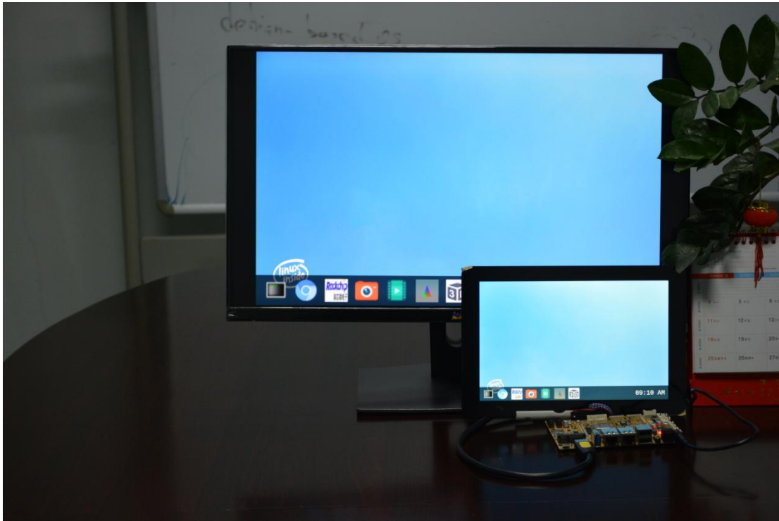
EM3568 supports both lvds and HDMI display.
