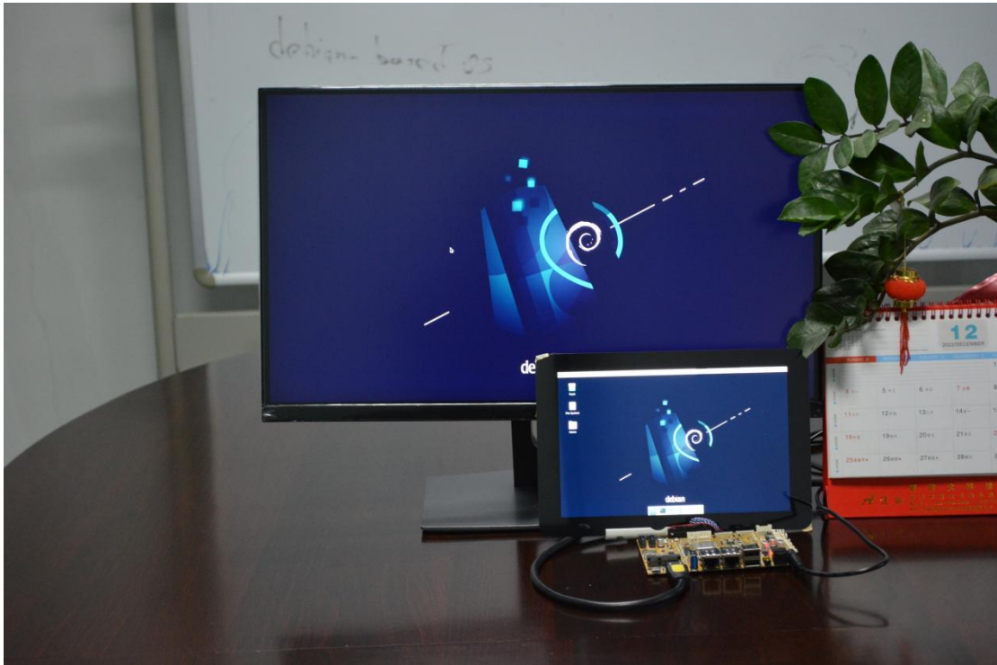
LVDS capacitive touch screen and HDMI default differential display.
